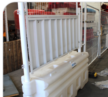
Half hoarding & fence next to vehicle gate
